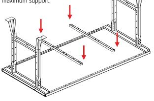
3. Attach the stringer (Ref. No. 2) to the rear legs, skipping the top two holes and using the next four holes from the top of each leg. NOTE: The legs are symetrical, so the front and rear of the bench will be determined by where you place the stringer. Attach with eight <sup>1</sup>/4"-20 x <sup>5</sup>/8" bolts, nuts, and lock washers (Ref. Nos. 18, 19, 20), four on each side.
