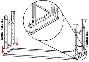
NOTE: When assembing a 96" workbench, the third leg should be mounted in the center of the top to reinforce the tops stability and allow for the load capacity.
